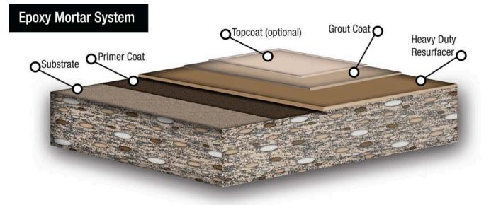
Epoxy Mortar Flooring System is a troweled, high strength concrete resurfacing material. It is used for environments requiring an industrial grade floor or when a concrete floor has sustained damage requiring a 3/16" to 1/4" surface restoration.
